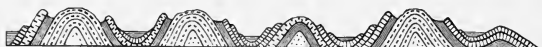
FIG. 134.—Section of the Jura Mountains, showing ridges following the anticlines and valleys along the synclines.
